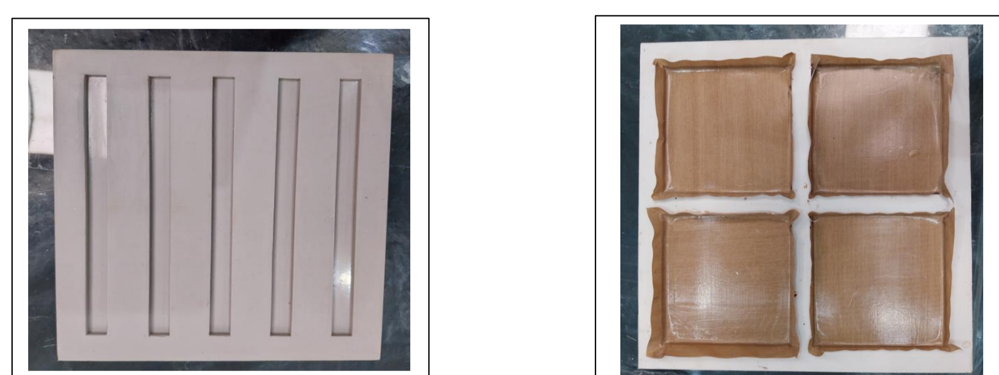
Figure 2. Silicon moulds. Right: LOI Test coupons; Left: Cone calorimeter coupons
