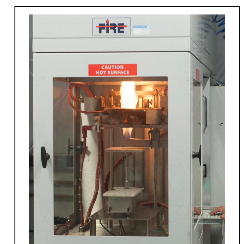
Figure 4. Cone Calorimeter Test
